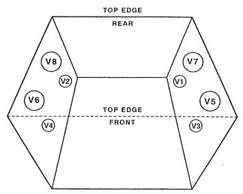
Diagram indicates relative positions of all (8) tubes located on two circuit boards as viewed from the front and looking down from above the amplifier.
